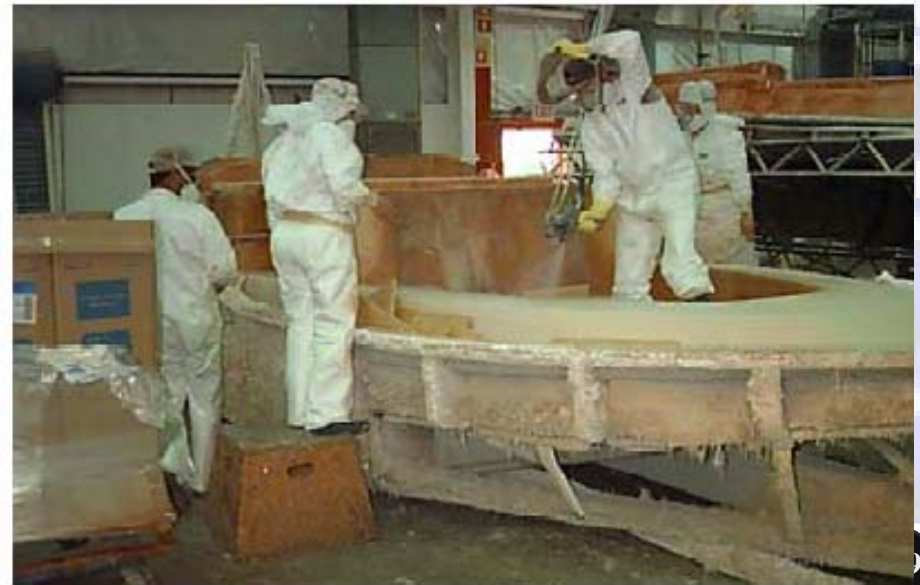
Conventional hand layup for boat building
