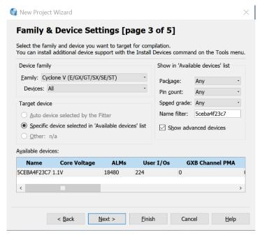
Figure 6. Set FPGA target
