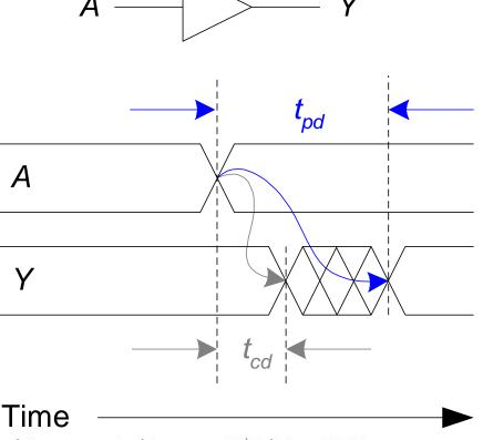
Note: Timing diagram shows a signal with a high and low and transition time as an 'X'.
