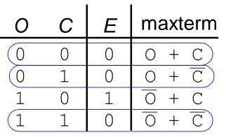
$E = (O + C)(O + \overline{C})(\overline{O} + \overline{C})$  $= \Pi(M0, M1, M3)$
