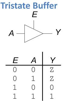
Note: tristate buffer has an enable bit (E) to turn on the gate
