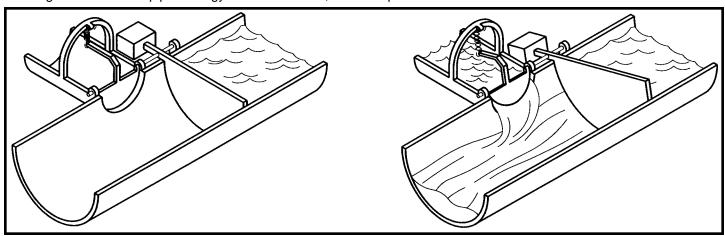
What would happen if the base and collector were connected together? Once there is enough pressure to overcome the spring in check valve DE (0.7V) there would be only slight resistance and no current gain. This situation should sound familiar since this is exactly how a diode operates. When the base and collector of a transistor are connected together the transistor becomes a diode.
