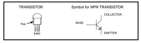
Note the small arrow in the emitter, this indicates which direction the current will flow through the device.
