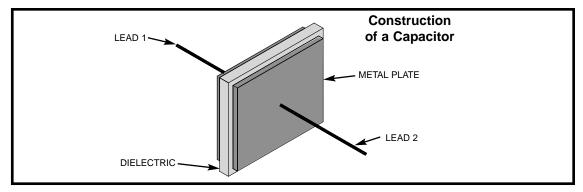
The dielectric is the material that holds the electric charge (pressure), just like the rubber diaphragm holds the water pressure. Some dielectrics may be thought of as stiff rubber, and some as soft rubber. The capacitance and working voltage of the capacitor is controlled by varying the number and size of metal-dielectric layers, the thickness of the dielectric layers, and the type of dielectric material used.
