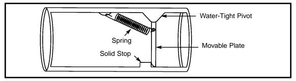
The check valve only allows water to flow in one direction, to the right in this drawing. There is a small spring and if the water pressure exceeds a certain level then the spring will be stretched and the valve opened. If the pressure is to flow to the left then the plate will be pressed against the solid stop and no water will flow.
