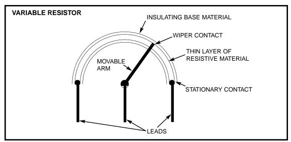
The dial on the variable resistor moves the arm contact and sets the resistance between the left and center pins. The remaining resistance of the part is between the center and right pins. For example, when the dial is turned fully to the left, there is minimal resistance between the left and center pins (usually  $0\Omega$ ) and maximum resistance between the center and right pins. The resistance between the left and right pins will always be the total resistance, ( $50k\Omega$  for your part).
