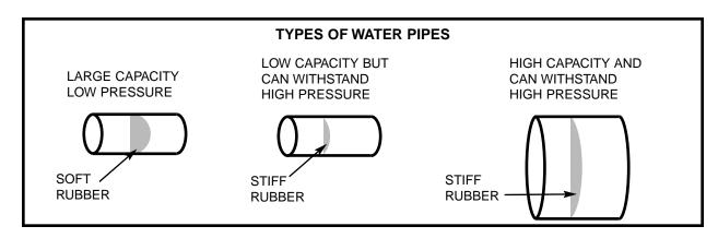
Similarly, capacitors are described by their capacity for holding electric charge, called their **Capacitance**, and their ability to withstand electric pressure (voltage) without damage. Although there are many different types of capacitors made using many different materials, their basic construction is the same. The wires (leads) connect to two or more metal plates that are separated by high resistance materials called **dielectrics**.
