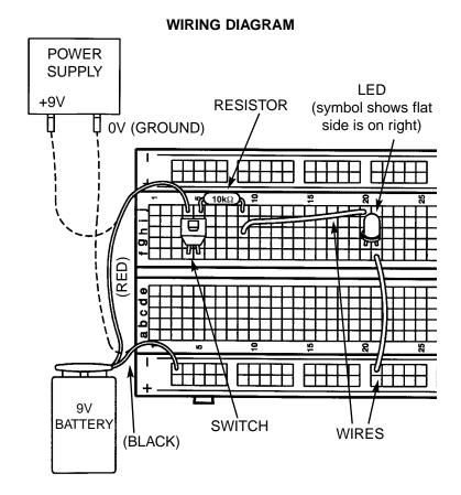
The Wiring Checklist and Wiring Diagram show you ONE way of connecting the circuit components using your breadboard. There are many other ways that are also correct. The important thing is that the electrical connections are as shown in the schematic (see below).
