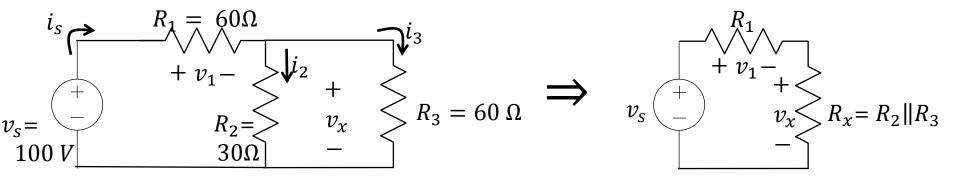
$$R_{\chi} = R_2 ||R_3| = \frac{R_2 R_3}{R_2 + R_3}$$
