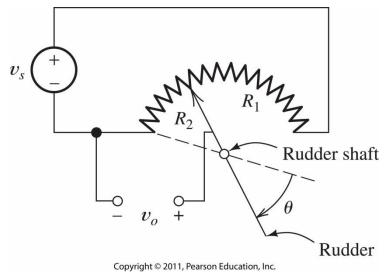
$$v_0 = v_s \frac{R_2}{R_1 + R_2} = \mathbf{K}\boldsymbol{\theta}$$
