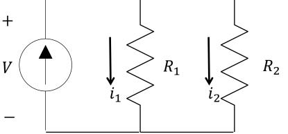
Smaller the resistor  $\rightarrow$  more current through parallel path
