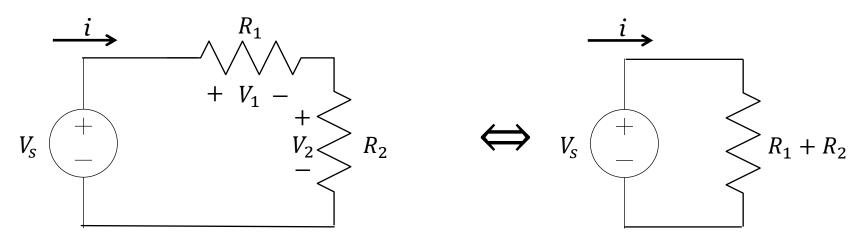
$\begin{aligned} v_1 &= iR_1 & v_2 &= iR_2 \\ &= V_s \left(\frac{R_1}{R_1 + R_2}\right) & = V_s \left(\frac{R_2}{R_1 + R_2}\right) \end{aligned} \qquad i = \frac{V_s}{R_1 + R_2} \end{aligned}$
