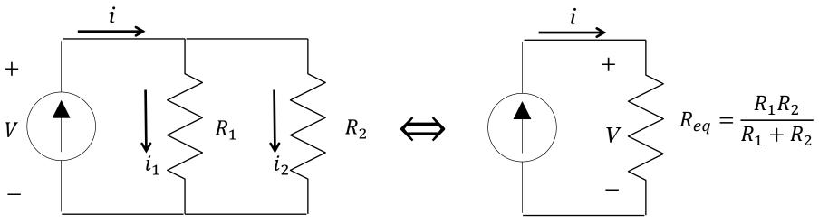
$$i_{1} = \frac{v}{R_{1}} = \frac{i}{R_{1}} \left( \frac{R_{1}R_{2}}{R_{1} + R_{2}} \right) \qquad i_{2} = \frac{v}{R_{2}} \qquad v = iR_{eq}$$
