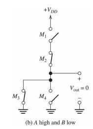
Only NMOS path connected *V*<sub>out</sub> is low
