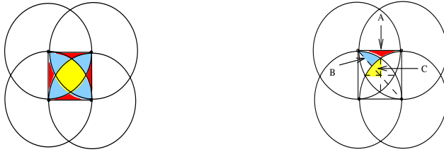
(a) Four sensors in a square arrangement (b) Selected areas A , B , and C
