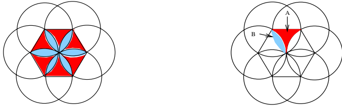
(a) Six sensors in a regular hexagon arrangement (b) Selected areas A and B
