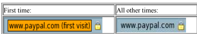
Figure 4. Visiting a SSL domain using Firefox for the first time (Figure taken from [4])
