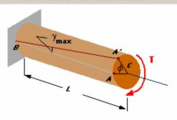
For a uniform shaft of radius  $\epsilon$  and length  $\ell$ , it has been shown that the maximum shearing strain  $\gamma_{\max}$  is related to the angle of twist  $\phi$  by
