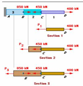
Determine the displacement of end D of the rod shown, knowing that it is made from a steel with E = 200 MPa.
