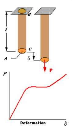
If the cross-sectional area is  $2\,\text{A}$ , a load of  $2\,\text{P}$  is required to produce the same deformation. In both cases the normal
