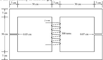
Solution This core can be divided up into five regions. Let  $\mathcal{R}_1$  be the reluctance of the left-hand portion of the core,  $\mathcal{R}_2$  be the reluctance of the left-hand air gap,  $\mathcal{R}_3$  be the reluctance of the right-hand portion of the core,  $\mathcal{R}_4$  be the reluctance of the right-hand air gap, and  $\mathcal{R}_5$  be the reluctance of the center leg of the core. Then the total reluctance of the core is
