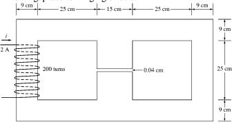
Solution This core can be divided up into four regions. Let  $\mathcal{R}_1$  be the reluctance of the left-hand portion of the core,  $\mathcal{R}_2$  be the reluctance of the center leg of the core,  $\mathcal{R}_3$  be the reluctance of the center air gap, and  $\mathcal{R}_4$  be the reluctance of the right-hand portion of the core. Then the total reluctance of the core is
