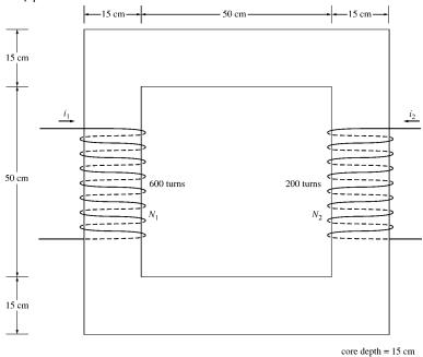
SOLUTION The two coils on this core are would so that their magnetomotive forces are additive, so the total magnetomotive force on this core is
