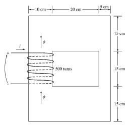
Solution There are three regions in this core. The top and bottom form one region, the left side forms a second region, and the right side forms a third region. If we assume that the mean path length of the flux is in the center of each leg of the core, and if we ignore spreading at the corners of the core, then the path lengths are  $l_1 = 2(27.5 \text{ cm}) = 55 \text{ cm}$ ,  $l_2 = 30 \text{ cm}$ , and  $l_3 = 30 \text{ cm}$ . The reluctances of these regions are:
