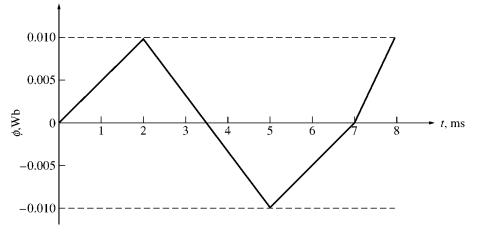
SOLUTION By Lenz' Law, an increasing flux in the direction shown on the core will produce a voltage that tends to oppose the increase. This voltage will be the same polarity as the direction shown on the core, so it will be positive. The induced voltage in the core is given by the equation
