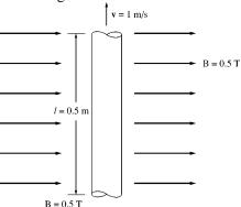
Solution The induced voltage on this wire can be calculated from the equation shown below. The total voltage is zero, because the vector quantity  $\mathbf{v} \times \mathbf{B}$  points into the page, while the wire runs in the plane of the page.
