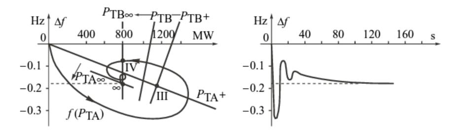
The variation in tie-line power interchange is similar to example 2, except that it settles down to 800 MW (instead of zero MW).
