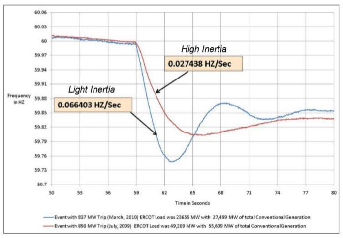
System inertia is the amount of kinetic energy stored in all spinning turbines and rotors in the system. System inertia decreases with more inverter-based generation, thus, Nadir will be lower with lower inertia.
