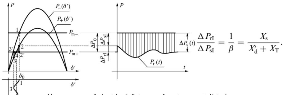
$X_s$ : measure of electrical distance of system w.r.t disturbance  $X'_d+X_T$ : measure of electrical distance of remaining gen. w.r.t disturbance
