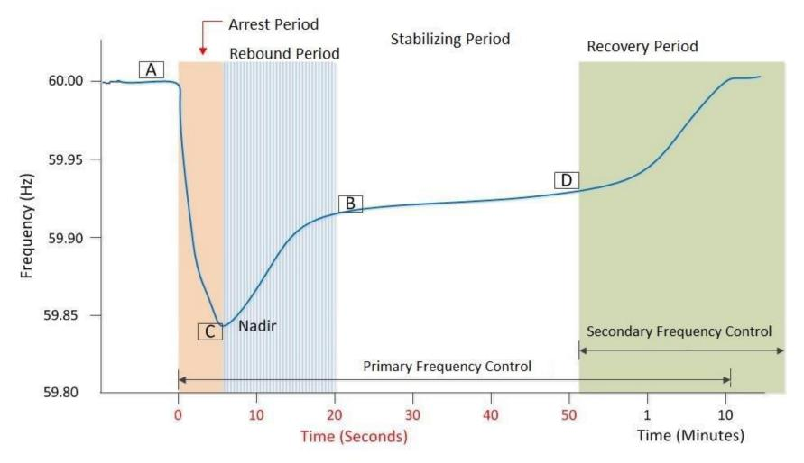
**Point A** - pre-disturbance frequency; **Point C** or Nadir - maximum deviation due to loss of resource; **Point B** - stabilizing frequency and; **Point D** - time the Balancing Authority begins the recovery from the loss of resource.
