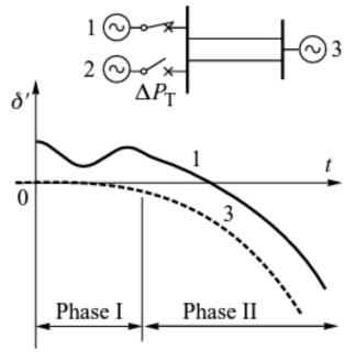
For the case of the network to the left, the contribution of the generator remaining in operation and the rest of the system in meeting the lost power:
