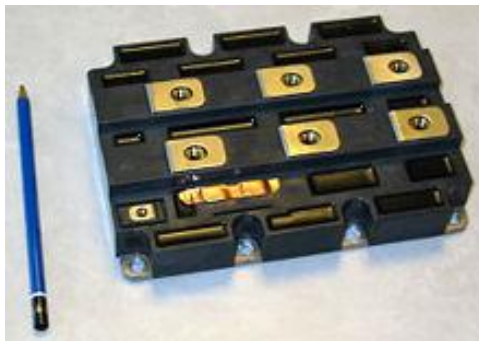
IGBT-Module with a rated current of 1.2 kA and a maximum voltage of 3.3 kV
