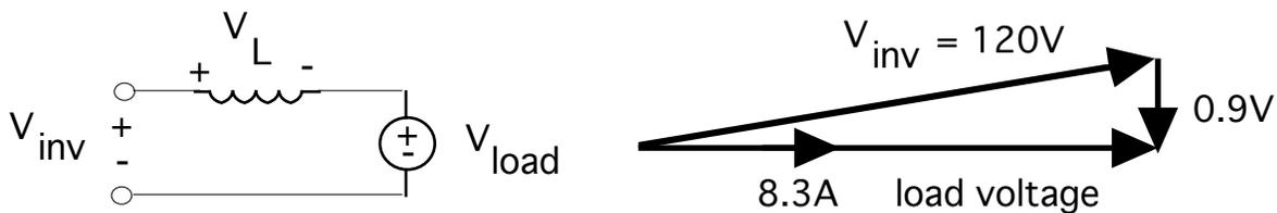
$$V_L = (8.3)(0.11) = 0.9\text{V} ; V_{\text{load}} = 120\text{V}$$
