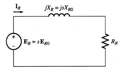
Now we can have the rotor equivalent circuit
