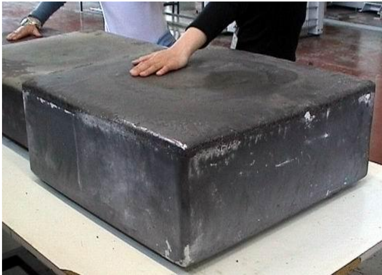
Slab of multi-crystalline silicon after growth.
