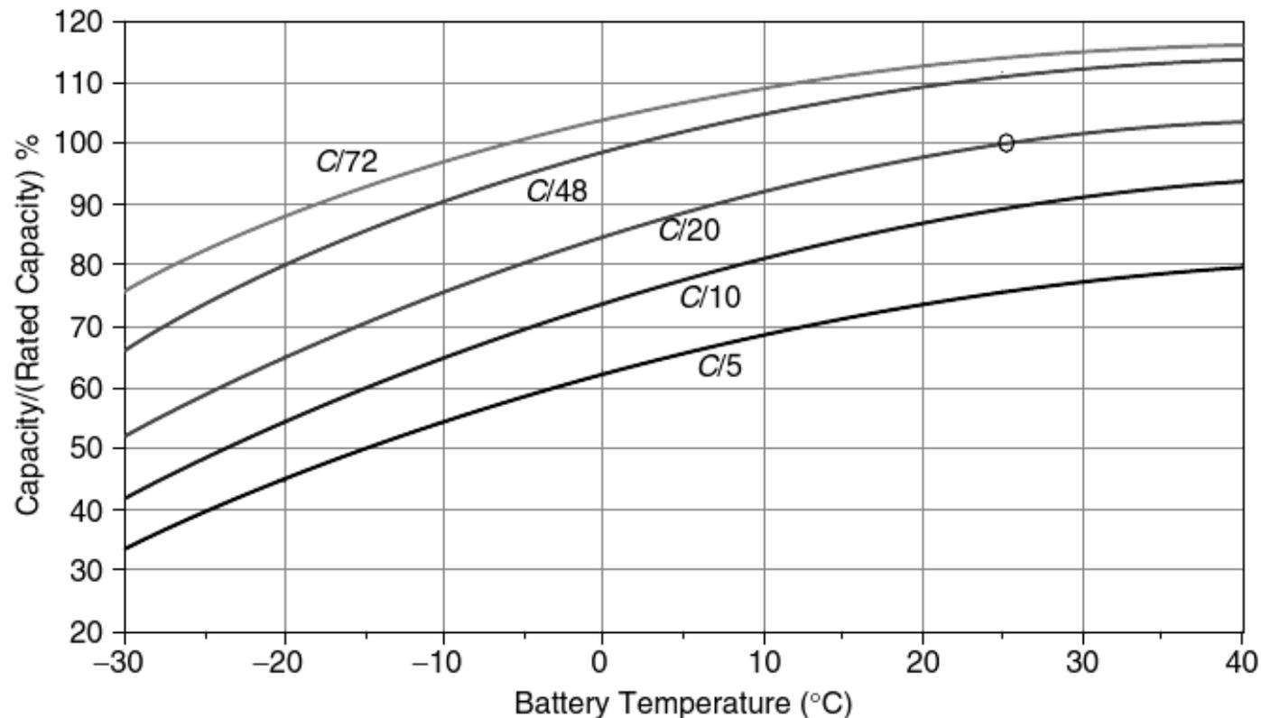
Ratio is based on a rated capacity at C/20 and 25°C
