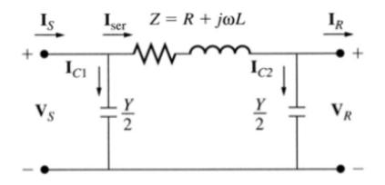
• The total series resistance and series reactance are calculated as before. Similarly, the total shunt admittance is given by
