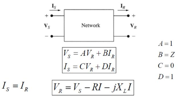
• The equation is similar to that of a transformer (w/o shunt impedance)
