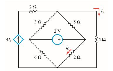
2) Determine the currents I' in the circuit below. Also calculate the power consumed by each resistor.
