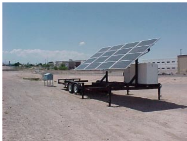
Fig. 1 1760 W PV powered air monitoring system
